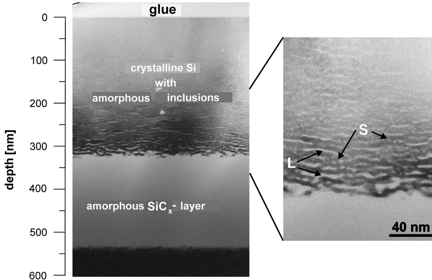
$180\text{keV } C^+ \rightarrow Si(100), 150^\circ\text{C}, 4.3 \times 10^{17}\text{cm}^{-2}$
