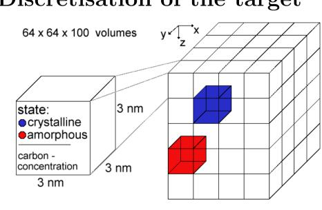
• divided into cells with a cube length of 3nm
