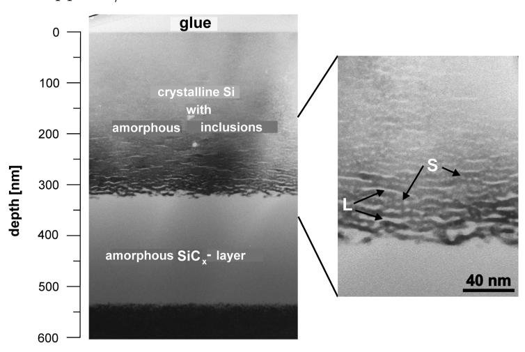
Cross-section TEM bright-field images:  $180 \ keV \ C^+ \to Si, \ T_i = 150 \,^{\circ}\text{C}, \ \text{Dose:} \ 4.3 \times 10^{17} \ cm^{-2}$ Amorphous inclusions appear white on darker backgrounds L: amorphous lamellae, S: spherical amorphous inclusions
