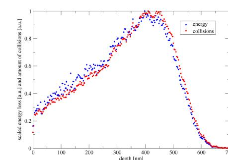
⇒ identical depth profiles for number of collisions per depth and nuclear stopping power
