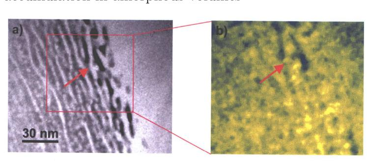
Bright-field TEM image and respective EFTEM C map:  $180 \, keV \, C^+ \to Si, \, T_i = 200 \, ^{\circ}\text{C}, \, \text{Dose: } 4.3 \times 10^{17} \, cm^{-2}$ yellow/blue: high/low concentrations of carbon
